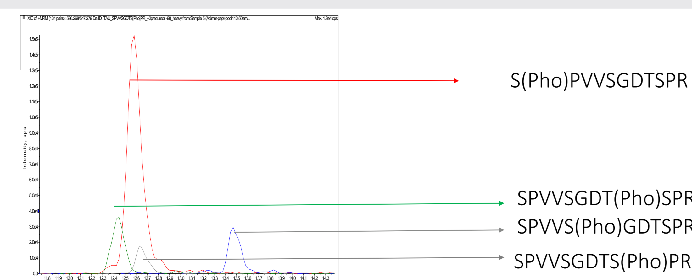
Figure 4 : LC-SRM chromatogram, allowing differentiation of mono-phosphorylated forms of SPVVS GDTSPR tau peptide.
